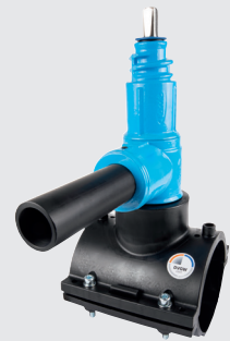
Service valve with milling device (punch) and electro-fusion saddle with horizontal PE fusion end (313-05)
