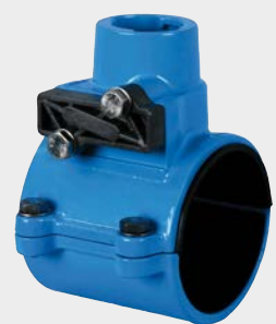
Tapping sleeve with auxiliary shut-off device: auxiliary shutting off by means of a shut-off blade of stainless steel, lateral drilling or drilling from top possible
