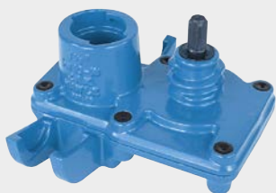
Pipe drilling saddle type Hawlinger®: drilling from above, shutting off via shut-off blade of stainless steel (see figure next page)
