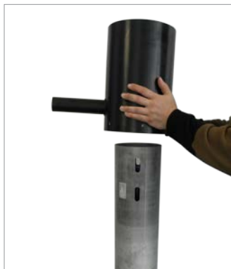
6. Apply commercial lubricant to the inner seal. Place the flood protection over the standpipe without the lid.
