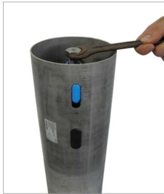
3. Loosen the centering screw.
