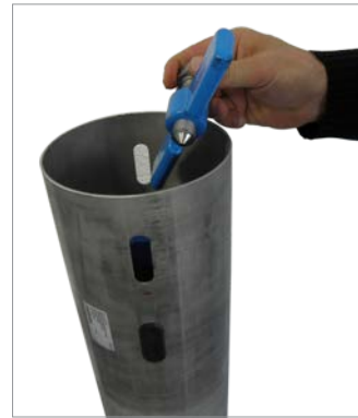
4. Dismantle the spindle holder.
