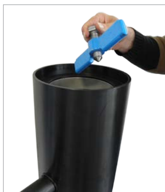
10. Place the spindle holder.
