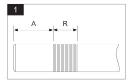
In case of pipes with very smooth surfaces (e.g. PE-X pipes) we recommend roughening the pipe end only in the area of the grip ring (see table) perpendicular to the pipe axis!
