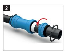
Remove the retaining ring. Unscrew the taper ring (blue cast iron ring) with locking key Ord. No. 609-00.
