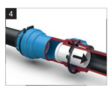
Check tensile strength and tightness by performing a pressure test.
